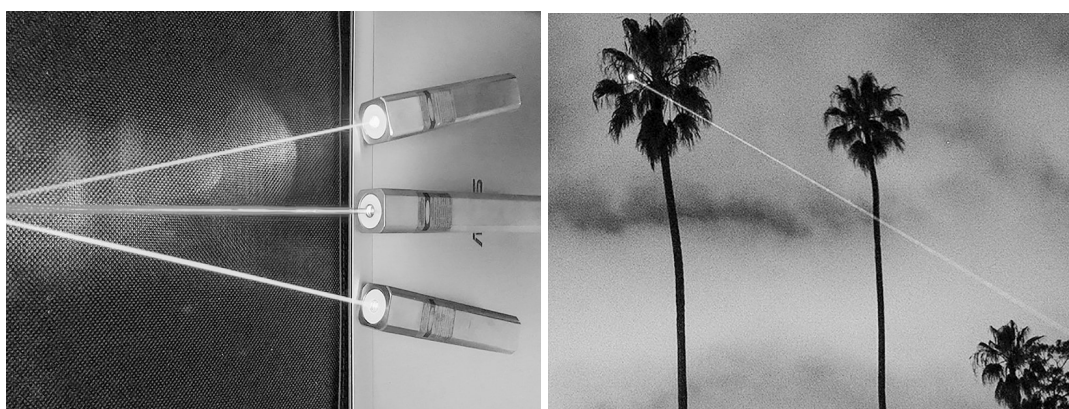
Hình 1: Red (635 nm), blueish violet (445 nm), and green (520 nm) laser pointers. A 5mW green laser pointer directed at a palm tree at night.
